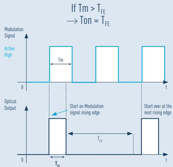
$T_m$  = Modulation input timing
